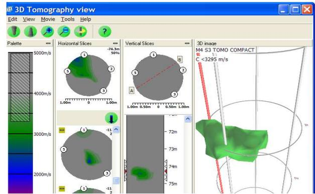
While regular (1D) CSL can only show the depth of an anomaly, tomography can help visualize its shape, size, and location. Tomography is an analysis and presentation method of captured CSL data that projects the logged results into a two-dimensional (2D) plane or three-dimensional (3D) body.
